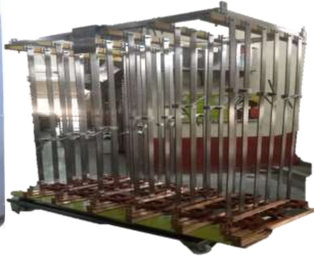
1700kW Sliding Type Load Bank, CESI LAB, Saudi Arabia
